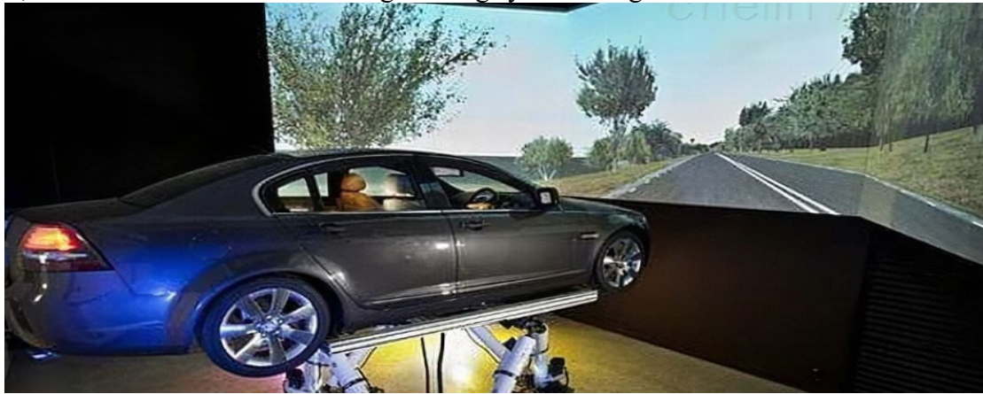
Figure 4 Projection visual simulation simulator.
